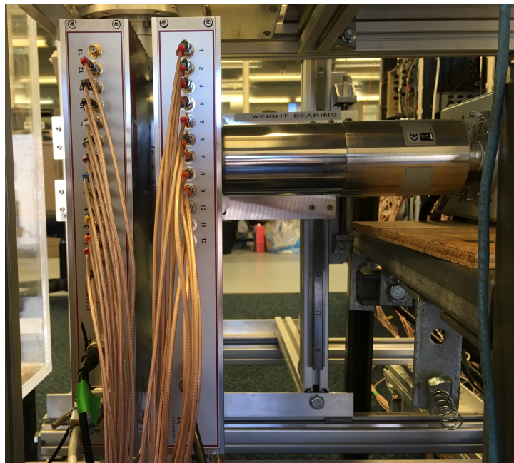
Figure 3.1: Photograph showing the side view of GRI+. The scatter detector, absorber detector and coaxial detector are displayed from left to right.
